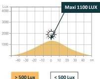
> 500 Lux < 500 Lux Measurement in Lux upwards at 50 cm from the light source :
