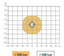
Measurement in Lux on the worktop in profile view at 35 cm:
