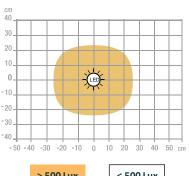
> 500 Lux < 500 Lux Measurement in Lux on the worktop in profile view at 35 cm:
