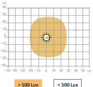
Measurement in Lux on the worktop in profile view at 35 cm:
