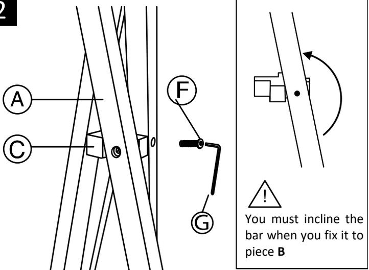
Joined the assembly of pieces **A** and **B** to the central piece **C**
