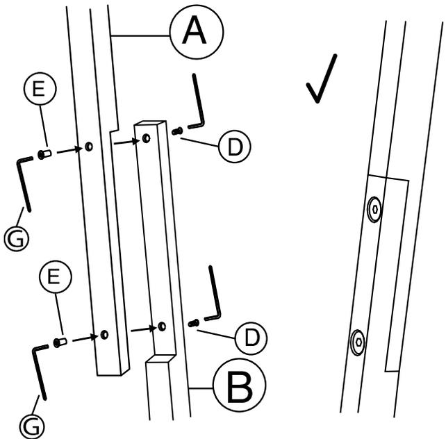
First, joined the two parts **A** and **B** together with the screws **D** and **E**. Do it with all the parts
