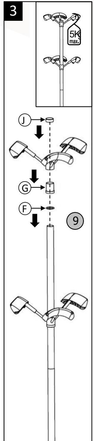
Diagram illustrating the third step of assembly: attaching the cap (J) to the top of the pole. An inset shows the final assembled product with a weight limit label indicating 5kg max.
