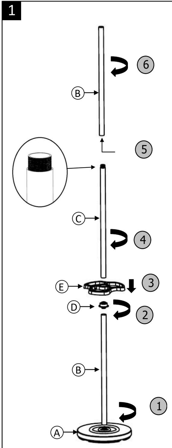
Diagram illustrating the first step of assembly: attaching the base (A) to the main pole (B). The pole is inserted into the base, and the sleeve (F) is slid onto the pole. The cap (D) is placed on the pole, and the bracket (E) is attached to the pole. The extension pole (C) is then inserted into the main pole (B).
