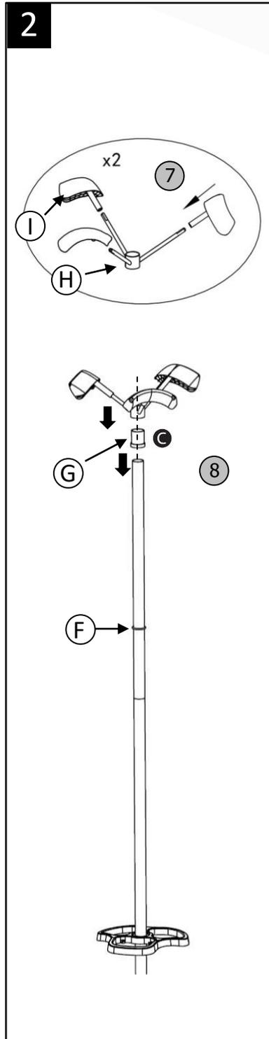
Diagram illustrating the second step of assembly: attaching the light heads (H) to the pole. The light heads are inserted into the mounting brackets (I) and secured with the connector (G). An inset shows a close-up of the light head being attached to the pole.
