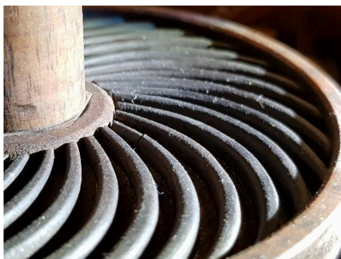
Figure 12 Sillons meule tournante
